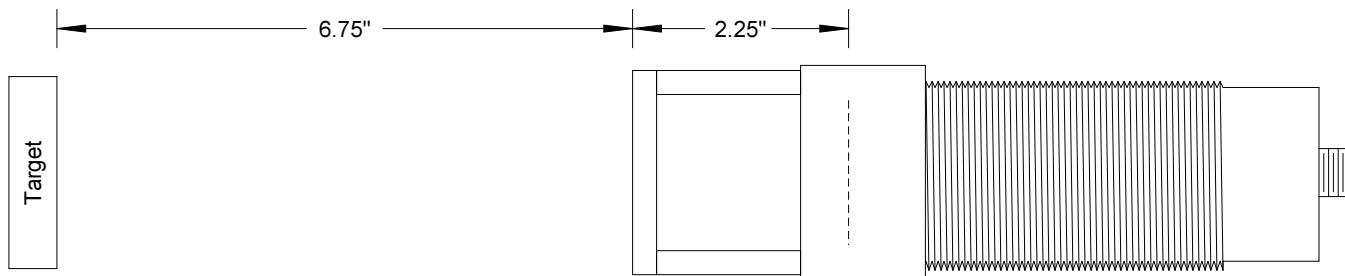
6. Calculate the voltage for the far distance. Add 2.25" to the measured distance and then multiply by the volts per inch. Adjust P2 for the calculated voltage.
